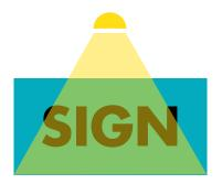
**Externally Illuminated Signs** are illuminated by a source of artificial light that is outside of the sign.
